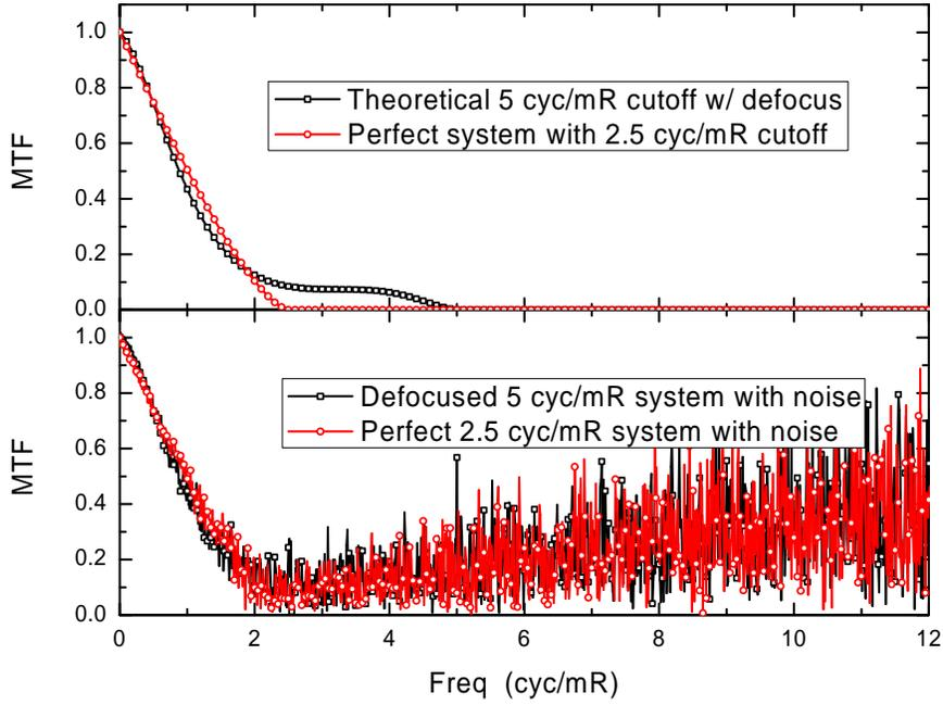
Fig. 1. The above shows plots of calculated MTF curves for two systems. The first is a system with a 5 cyc/mR cutoff, without aberrations but with a defect of focus of  $\frac{1}{2}$  wave. The second is an ideal system with a 2.5 cyc/mR cutoff. The upper plot shows the calculated theoretical MTF for the two systems. The lower plot shows the calculated MTF after the addition of a Gaussian noise distribution to the ESF used to derive the MTF.
