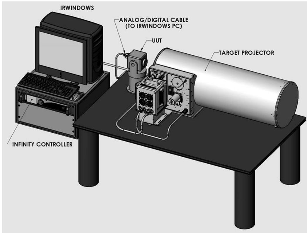
Figure 3 Standard IR test bench configuration
