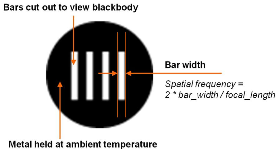
Figure 2 A 4-bar target sets the spatial frequency and uses a blackbody to set temperature difference
