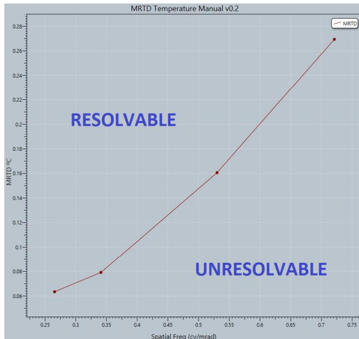
Figure 1 MRTD plot, temperature vs. spatial frequency
